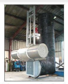
Cylinder screen can be adapted for vertical pump applications. Note the docking inlet with trash rack at bottom of wet well pipe.
