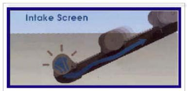
Screen rolls down the track to docking inlet at bottom. Water flows through the screen & up the pump column to the pump discharge
